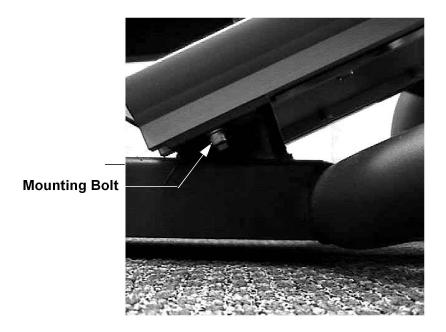
6. Remove the two mounting bolts from the front bottom of the ramp assembly.
